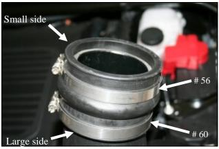
**CAB** tube. Loosely install the #56 Hose Clamp on the small side of the Hump Hose, and the #60 Hose Clamp 1) on the Large side. (B) Slide the Hump Hose and Clamps downward on the tube, creating a compact assembly as shown.
