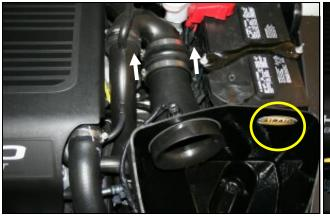
11. A.) Place the CAB in the original location of the 12.Install the Airaid Premium Filter onto the Filter adapt-Factory Air box and secure using the factory hardware er and tighten the clamp. from step 4. B.) Slide the coupler and clamps onto 90 deg. Elbow pipe and tighten the clamps. C.) Reconnect the Air Temperature Sensor. Apply the Airaid Decal inside of the Airbox as shown.
