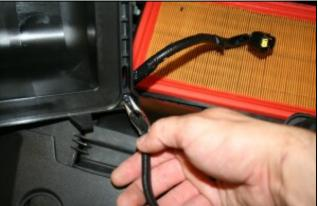
the fins of the wiring harness anchor and pull it out of the air box lid.
