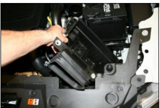
4. A.) Using an 8mm socket, remove the two factory 5. Remove the factory air box assembly from the vehicle. 6. Prepare the Filter Adapter for installation by position-
