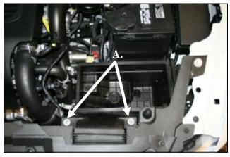
air box bolts and set aside. The will be reused in step 11. **B.**) Remove the factory air filter element.
