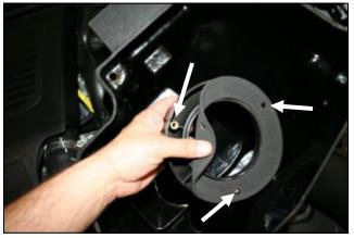
ing the Adapter Gasket on the mounting side and lining up the holes.
