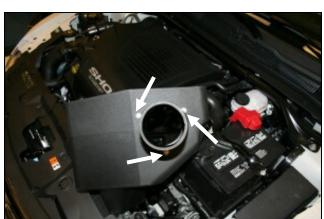
7. Install the Filter Adapter to the inside of the Cool Air 8. A) Install the Hump Hose, large side first onto the 9. Remove the Air Temperature Sensor from the factory Box, CAB using the three 1/4"-20 hex head bolts and 1/4" flat washers as shown.
