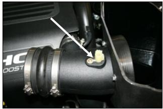
10. A) Transfer the factory Air Temperature Sensor into the Airaid Intake tube and align the sensor tab with the Groove in the tube. B) Secure the sensor to the tube using the 8-32 Button Head Bolt and the 3/4" washer.
