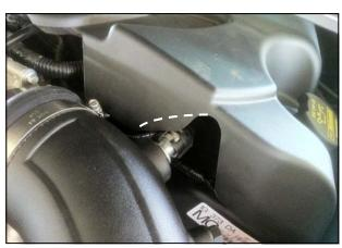
For Performance Package equipped motors, it is recommended that the installer enlarge the breather cut out in the engine cover using a Dremel with a cut off wheel, then de burr for a professional look.
