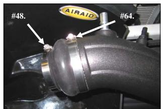
7. Slip the Hump Hose (#4) and Hose clamps onto the 8. Insert the Intake Tube into the CAB first, then lower Airaid Intake Tube. Slide the #64 Hose Clamp (#10) onto the Tube down and onto the throttlebody. Tighten the the tube side and the #48 Hose Clamp (#9) onto the En- Hose Clamps. gine side. Leave the Hose Clamps loose for now.
