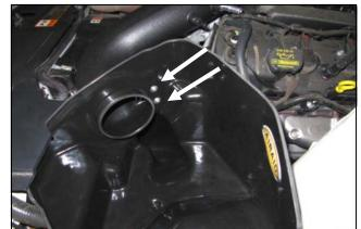
9. Secure the Intake Tube to the CAB using the two 1/4" Button Head Bolts (#6) and 1/4" Washers (#7).
