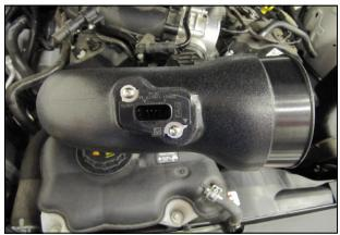
**5.**Transfer the **MAF** sensor into the Airaid Intake Tube (#2) and secure using the supplied 8-32 Button Head
