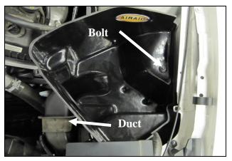
**4.** Install the **CAB** into the vehicle. Make sure that the Air inlet of the CAB mates with the factory duct, and the two locating cones on the bottom mate with the factory grommets. Next reinstall the factory bolt that was removed in step #3 through the steel sleeve and grommet and into the inner fender.
