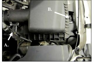
2. A) Slide the red lock tab back, and disconnect the wiring harness from the Mass Air Flow sensor (MAF). Carefully pry the harness anchor from the air box using a screwdriver. B) Using a 10mm socket, remove the bolt securing the air box to the inner fender and remove the air box assembly. This bolt will be reused in step 4.
