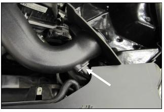
**11.** Reconnect the Mass Air Flow sensor. Slide the locking tab back into the connector.
