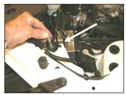
**6.** With a 10mm socket, remove and save the bolt from the anti-lock brake bracket. It will be re-installed later in step #8.
