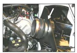
**10.** Install the hump hose (#5) on the filter adapter (#6), with two #72 hose clamps (#13). Tighten <u>only</u> the clamp next to the **CAD**.
