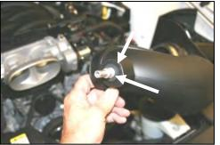
**11.** Install the supplied grommet (#14) and aluminum fitting (#17) into the Airaid intake tube as shown.
