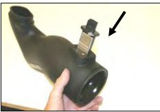
**13.** Align the two slots in the tubes, and install the factory mass air sensor removed from step #5. Make sure the screw holes line up, then install the two supplied button head screws. (#12). **DO NOT USE THE FACTORY SCREWS!!**
