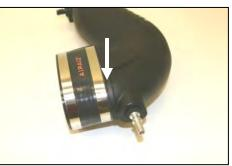
**14.** Install the oval coupler (#4) with two #72 hose clamps (#13). Tighten <u>only</u> the clamp closest to the aluminum fitting. (*Hint: For a clean look, locate the hose clamp tightening screws under the tube*)!
