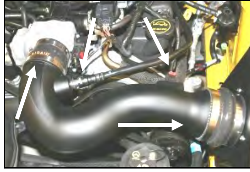
14. Install the Airaid Intake Tube into the hump hose first, and then into the reducing coupler, adjust for fit, and then tighten the four hose clamps. Reconnect the breather hose, and the wiring harness to the MAF sensor.
