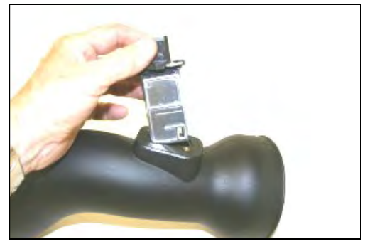
12. Install the MAF sensor from step #5 into the Airaid Intake Tube. Use the two supplied 8-32 button head screws (#10), to securely fasten the MAF sensor. Do Not Use The Factory Screws!
