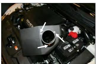
7. Install the Filter Adapter to the inside of the Cool Air Box, CAB using the three 1/4"-20 hex head bolts and 1/4" flat washers as shown.
