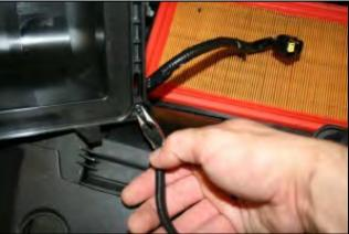
**3.** Using a pair of needle nose pillars, carefully compress the fins of the wiring harness anchor and pull it out of the
