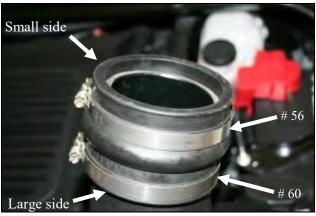
8. A) Install the Hump Hose, large side first onto the CAB tube. Loosely install the #56 Hose Clamp on the small side of the Hump Hose, and the #60 Hose Clamp 1) on the Large side. (B) Slide the Hump Hose and Clamps downward on the tube, creating a compact assembly as shown.
