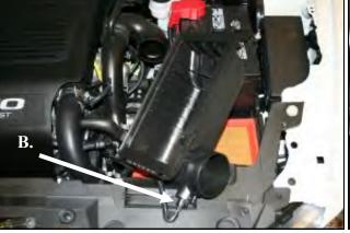
2.A.) Unfasten the factory air box clips and separate the upper half of the air box from the intake assembly. **B.**) Disconnect the air temperature sensor.
