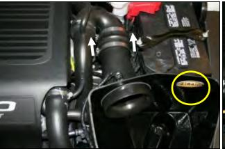
11. A.) Place the CAB in the original location of the Fac- 12. Install the Airaid Premium Filter onto the Filter adapttory Air box and secure using the factory hardware from er and tighten the clamp. step 4. B.) Slide the coupler and clamps onto 90 deg. Elbow pipe and tighten the clamps. C.) Reconnect the Air Temperature Sensor. Apply the Airaid Decal inside of the Airbox as shown.
