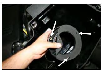
4. A.) Using an 8mm socket, remove the two factory air 5. Remove the factory air box assembly from the vehicle. 6. Prepare the Filter Adapter for installation by positioning the Adapter Gasket on the mounting side and lining up the holes.
