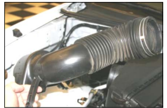
3. Remove the complete intake tube from the vehicle.
