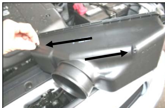
8. Install the two rubber washers (#17) onto the two plastic plugs (#16) that are provided in the hardware kit, and insert them into the two weep holes in the factory air cleaner cover removed in step #4, as shown
