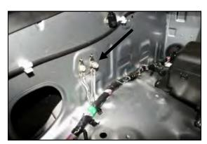
**5.** Remove the rear ground anchor bolt from the side of the fender well and save it for reuse in
