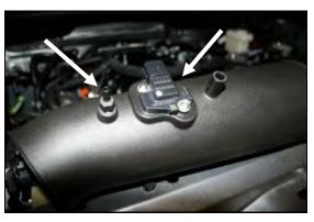
9. Re-install the MAF sensor into the Airaid intake tube (#2) as shown <u>using the supplied 8-</u> <u>32x3/8" button head screws (#12).</u> <u>Do Not Use The Factory Screws!</u> Next install the 1/8NPTx3/16" barbed fitting (#20) into the Airaid tube.
