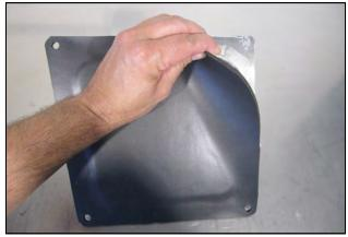
**10.** Prepare the Airbox Lid for Gasket installation by cleaning the mounting surface using a Prep Solvent or equivalent. Remove the adhesive backing from the Gasket and carefully apply it as shown with the screw holes aligned.
