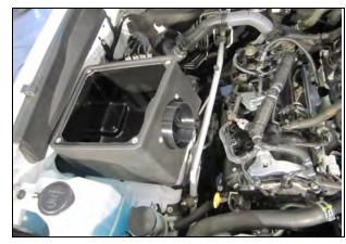
**12.** Position the Airaid Airbox assembly into the engine compartment as shown.
