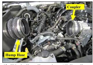
**13.** Slide the Hump Hose and two #68 Hose Clamps onto the Filter Adapter as shown. Slide the Coupler and the #48 and #64 Clamps on to the throttlebody. Leave the Clamps loose for now.
