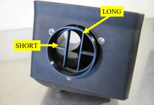
8. Install the Filter Adapter onto the Airbox using three sets of 1/4-20 Button Head Screws and Flat Washers. Note the positioning of the Adapter in the Airbox. When properly installed, the long air vanes are vertical and the short vanes are horizontal.
