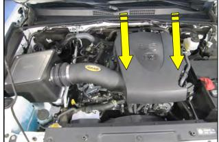
**21.** Reinstall the engine cover. Slowly lower the hood to test clearances. Make sure all clamps, hoses, bolts, and screws are tight. Double check the hood clearance. Reconnect the negative battery terminal.
