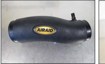
7. Install the Barbed fitting into the Airaid Intake Tube as shown. Apply the Airaid Badge to the Intake Tube as shown.
