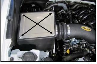
**19.** Remove the protective film from the other side of the Lid and mount the Lid onto Air Box using four  $1/4-20 \times 1/2$ " Button Head Bolts , and 1/4" Flat Washers .
