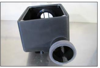
9. Prepare the Airbox inlet for Weatherstrip installation by cleaning the surface using a Prep Solvent or equivalent. Apply the self adhesive, Foam Weatherstrip onto the air inlet on the Air Box as shown. Trim any excess.
