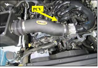
**14.** Insert the Intake tube into the Hump Hose and coupler. Align the tube with the PCV line, re connect it and tighten all 4 Clamps.
