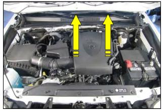
1. Disconnect The Negative Battery Terminal. Remove the engine cover. Lift up on the front of the engine cover to unseat the mounting grommets and remove it from the vehicle.
