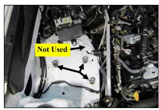
**11.** Install the three CAB Mounts, hand tight, into the weld nuts on the inner fender as shown. Note: One of the original air box mounting holes is not re used.
