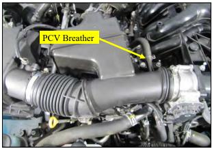
3. Disconnect the PCV breather line. Loosen the clamps on both ends of the intake tube and remove the entire intake/resonator assembly from the vehicle.
