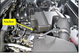
2. Pry the wire harness anchor from the tab on the resonator.
