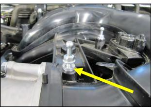
**20.** Remove the front engine cover mounting post and place the Aluminum Spacer onto the threaded stud like a washer and re tighten.
