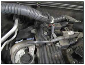
8. Secure the vacuum switching valve to the valve cover using one of the factory plenum bolts.
