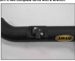
14. Remove the mass air sensor from the factory air filter housing and then install it into the AIRAID® intake tube and secure with the provided hardware.
