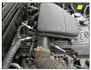
4. Remove the two bolts that secure the intake plenum to the valve cover, then remove the two bolts that secure the vacuum switching valve to the intake tube and disconnect the crank case vent hose from the valve cover.
