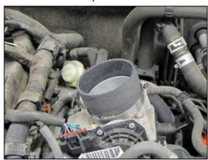
15. Install the coupler hose (084036) onto the throttle body and secure with the provided hose clamp.
