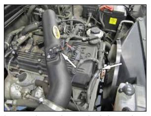
19. Connect the mass air sensor electrical connection and secure the wiring harness with the provided tie wrap.
