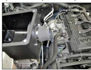
16. Install the coupler hose (084079) onto the filter adapter and secure with the provided hose clamp.
