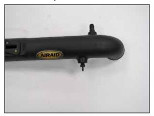
13. Install the provided vent fittings and AIRAID® decal onto the AIRAID® intake tube as shown.
