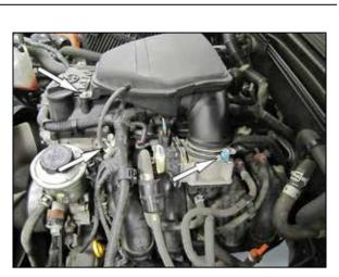
5. Remove the bolt securing the intake plenum to the valve cover, then disconnect the vent line from the fuel pressure regulator and loosen the hose clamp securing the intake plenum to the throttle body. Remove the intake plenum from the vehicle.
