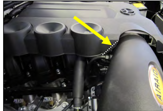
13. Place the engine cover back on top of the motor and note the location where it comes in contact with the Airaid Intake Tube. Remove the cover and trim the edge approximately 1/8" and reinstall.
