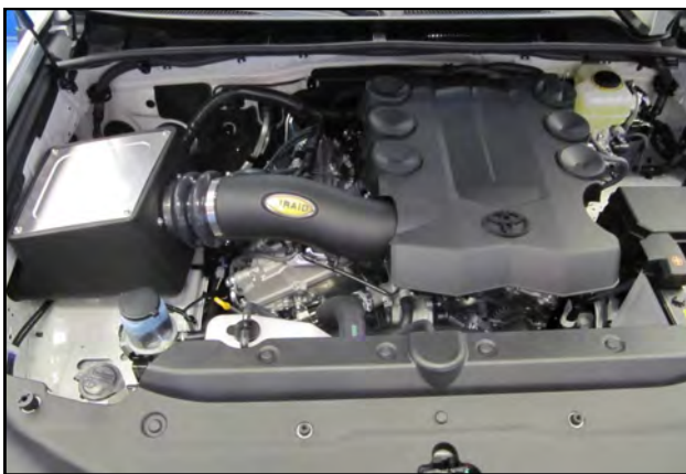
16. Double check your work! Make sure there is no foreign material in the intake path. Make sure all clamps, hoses, bolts, and screws are tight. Double check the hood clearance! Reconnect the negative battery cable!
