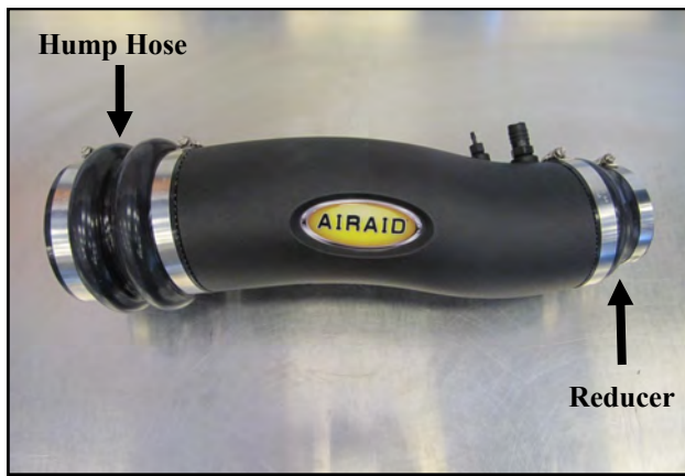
10. Slide the hump hose, and two #72 hose clamps onto the intake tube as shown. Slide the reducing coupler and the #48 and #64 clamps on the other end of the intake tube. Leave the clamps loose for now.
