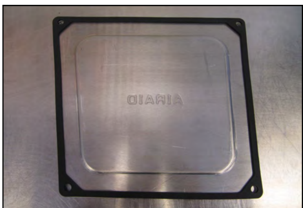
15. Place the gasket onto the underside of the air box lid and peel off the protective film. Mount the lid on the air box using four 1/4-20 x 1/2" button head bolts, and 1/4" flat washers.
