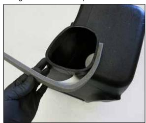
15. Install the foam inlet seal around the AIRAID fresh air inlet.
