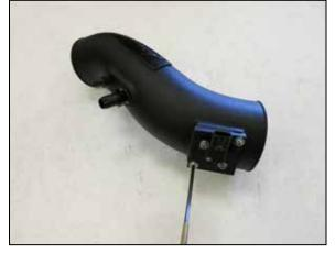
12. Install the MAF sensor assembly into the intake tube and secure with the provided hardware.
