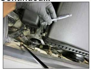
7. Loosen the rear air filter housing mounting bolt.
