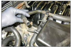
3. Disconnect the CCV vent hose and fuel pressure vent line from the plenum.
