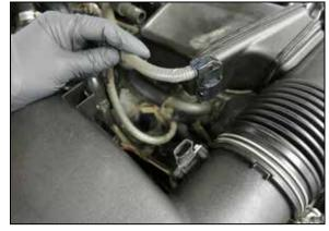
4. Disconnect the MAF sensor electrical connection and unhook the wiring from the air filter housing.
