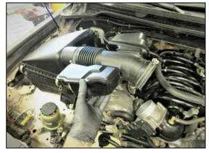
8. Remove the complete factory intake system from the vehicle.
