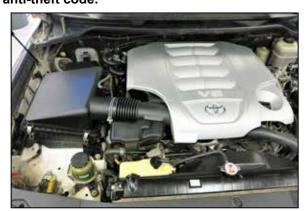
2. Lift off the engine cover and set aside.
