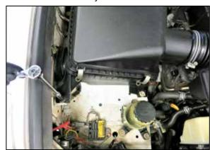
6. Loosen the two front air filter housing mounting bolts.
