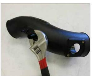
10. Install the provided vent fittings into the AIRAID intake tube as shown.
