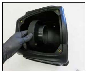
14. Install the filter adapter into the AIRAID filter housing and secure with the provided hardware.
