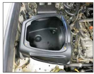
17. Install the AIRAID air filter housing into the vehicle and secure to the factory filter housing mounting location with the provided hardware.
