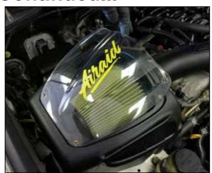
22. Install the AIRAID air filter housing cover and secure with the provided hardware.
