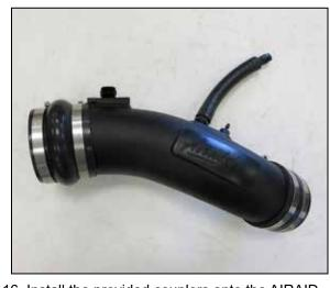
16. Install the provided couplers onto the AIRAID intake tube using the provided hose clamps.
