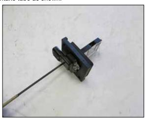
11. Remove the MAF sensor from the factory air filter housing and install it into the provided filter adapter with the hardware provided. Then install the provided gasket onto the bottom of the adapter.
