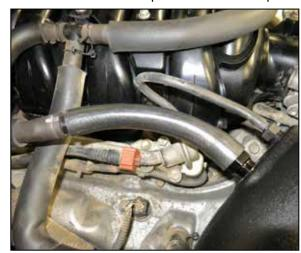
19. Connect the CCV hose and fuel pressure regulator vent hose.
