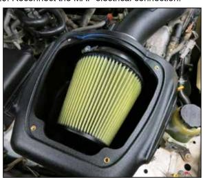
21. Install the air filter onto the adapter and secure with the provided hose clamp.
