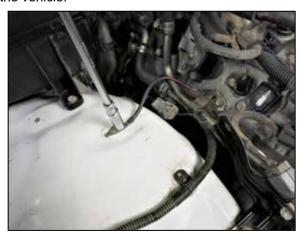
9. Remove the bolt that secures the engine ground to the inner fender.
