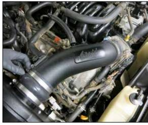
18. Install the intake tube assembly onto the throttle body and filter adapter, adjust for best fit and then secure with the provided hose clamps.
