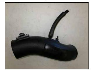
13. Install the provided CCV hose and fitting onto the intake tube as shown.
