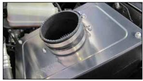
13. Install the provided step coupler onto the filter adapter and secure with the provided hose clamp.
