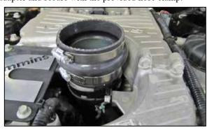
14. Install the provided hump coupler onto the turbo inlet and secure with the provided hose clamp.
