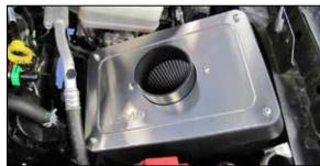
12. Install the lid assembly onto the AIRAID® air filter housing and secure with the provided hardware.
