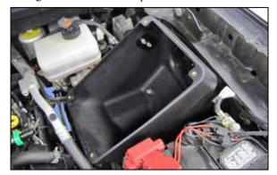
9. Install the AIRAID® air filter housing onto the mounting studs on the inner fender and secure with the factory bolt removed in step #4.
