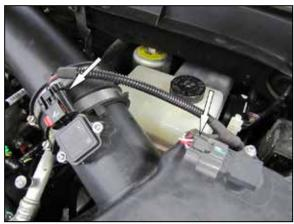
2. Disconnect the mass air sensor and inlet air temperature sensor electrical connections.
