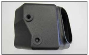
6. Remove the two mounting grommets from the factory lower air filter housing and install them into the AIRAID® housing as shown.
