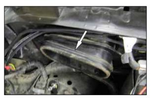
5. Remove the gasket from the factory fresh air intake.
