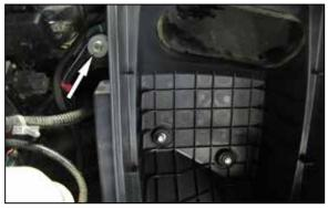
4. Remove the bolt that secures the lower air filter housing to the inner fender and then pull firmly up to release the lower housing from the mounting grommets and remove it from the vehicle.
