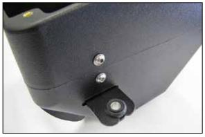
8. Install the grommet and sleeve from the previous step into the provided mounting bracket, then install the mounting bracket through the AIRAID® air filter housing and secure with the provided hardware.
