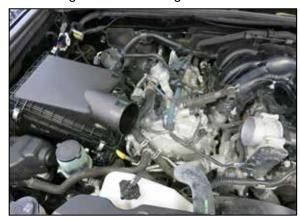
3. Disconnect the CCV hose and fuel pressure regulator vent line from the factory intake tube. Loosen the hose clamps that secure the factory intake tube and remove the tube from the vehicle.
