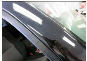
20. Use a 3/16" drill for the "A" pillar mounting bracket holes. Go slow and do not push hard while drilling to prevent drill bit wonder. Use tape or vacuum hose to create a 5/8" stop on the drill bit so the drill will only go 5/8" past the outer sheet metal.
