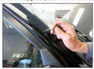
21. Use touch up paint to paint the raw sheet metal to prevent corrosion.
