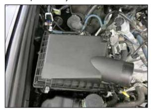
31. Reinstall the upper housing and air filter, secure with the factory over center clamps.
