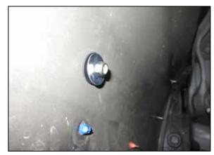
25. Secure the snorkel to the fender using the nuts and fender washers provided.
