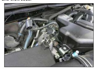
2. Disconnect the mass air sensor electrical connection and unhook the harness from the air filter housing. Remove the engine cover.
