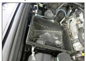
30. Reinstall the lower housing so the inlet goes into the snorkel hose. Secure with the provided hose clamp and factory hardware.
