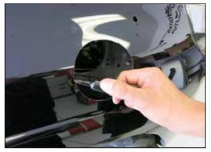
17. Use touch up paint or similar paint to paint the raw metal to prevent corrosion.
