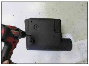
33. If you are installing this kit onto a vehicle equipped with an AIRAID intake kit, drill two 3/8"drain holes into the bottom of the AIRAID filter housing.
