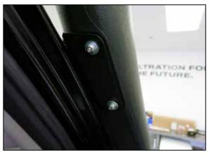
26. Secure the snorkel to the "A" pillar bracket with the hardware provided.
