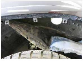
6. Carefully Pull back the inner fender to release the tabs enabling the inner fender to be pulled down to allow access behind the fender. **NOTE:** Replacement black screw grommets are provided incase the factory grommets break.
