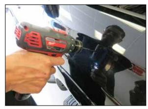
14. Once all the holes to be drill are marked, drill a 1/8" pilot hole for each hole.
