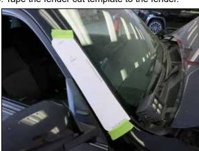
10. Tape the "A" pillar template onto the pillar.
