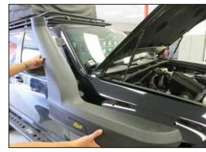
24. Install the snorkel onto the fender.
