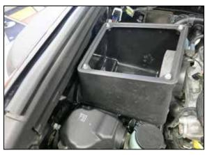
35. Reinstall the AIRAID filter housing and secure with the hose clamp and hardware provided.
