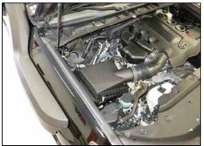
32. Reinstall the factory intake tube, reconnect the CCV and vent hoses, reconnect the mass air sensor electrical connection and reinstall the engine cover.
