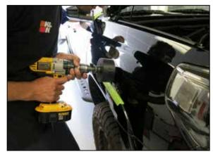
16. Drill the hole for the snorkel outlet with a 4-1/4" hole saw. Deburr the hole.
