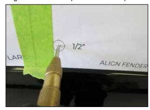
12. Us a center punch or similar device to mark the center of all the  $\frac{1}{2}$ " holes to be drilled.
