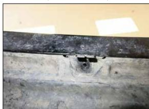
28. Reinstall the inner fender and secure with the factory hardware. **NOTE: Replacement black** screw grommets are provided incase the factory grommets break.
