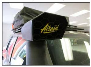
36. Install the snorkel scoop onto the Snorkel and secure with the provided hose clamp.
