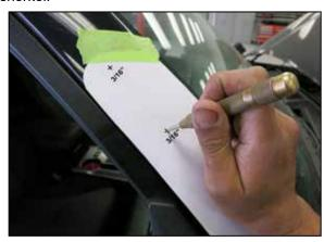
19. Temporarily install the snorkel onto the fender with the "A" pillar mounting bracket installed onto the snorkel. Check the alignment of the hole position of the template to the bracket and adjust as necessary. Remove the Snorkel assembly from the fender. Using a Center punch to mark the center of the holes to be drilled. **NOTE: Use patience and double check the alignment of the template before marking the holes to be sure they are in the correct position.**
