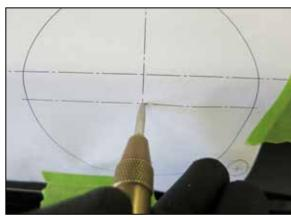
13. Us a center punch or similar device to mark the center of the 4-1/4" hole to be drilled.
