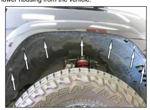
5. Remove the bolts that secure the inner fender well to the fender.
