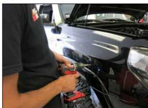
15. Drill the  $\frac{1}{2}$ " holes with a  $\frac{1}{2}$ " drill bit. Deburr the holes.
