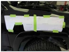
9. Tape the fender cut template to the fender.
