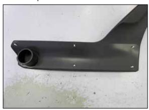
18. Install the provided M8 studs onto the snorkel and then apply gasket material to the back of the snorkel.
