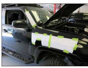
11. Verify the templets are positioned correctly using the text and lines printed on the template.
