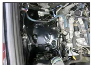
4. Release the over-center clamps that secure the upper air filter housing and then remove the upper housing. Remove the bolts that secure the lower housing to the inner fender and then remove the lower housing from the vehicle.
