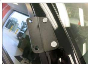
23. Install the snorkel bracket onto the "A" pillar using the provided rivets.
