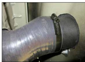
27. Install the coupling hose through the hole in the inner fender and connect it to the snorkel outlet. Secure with the provided hose clamp.
