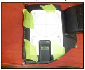
30. Cut out the lid drill template and tape onto the air filter housing lid as shown.
