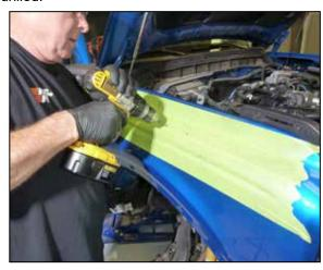
13. Drill a 1/8" pilot hole for all seven holes then drill the five mounting holes with a  $\frac{1}{2}$ " drill.
