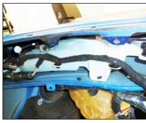
25. Reinstall the windshield washer bottle using the factory hardware. Secure the wiring harness to the bottle. Reinstall the filler neck using the factory hardware.
