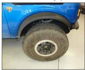
27. Reinstall the inner fender and secure with the factory bolts. If equipped, reinstall the extended fender flare and secure with the factory quarter turn fasteners, reinstall the wheel and secure with the factory lug nuts torqued to the proper specifications.
