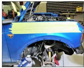
10. Apply painters' tape to the fender to protect the surrounding paint while drilling holes.
