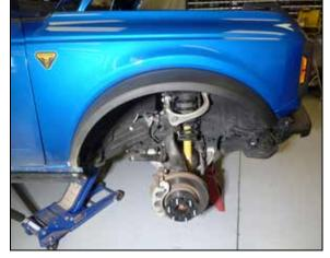
2. Jack up the front passenger side of the vehicle and support with a jack stand. Remove the front
