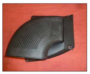
37. If installing this system onto a vehicle that is equipped with a K&N intake system, Install the snorkel adapter onto the provided K&N air box lid using the provided hardware.
