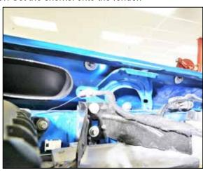
22. Install the three nuts onto the mounting studs along with the fender washers. Do not tighten the nuts.
