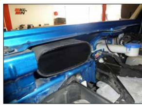
34. Slide the provided coupler all the way onto the snorkel outlet.
