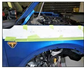
11. Install the assembled drill pattern onto the inner fender, the template needs to be placed accurately so the holed are placed in the proper location.
