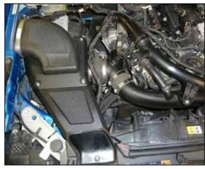
38. Install the lid onto the K&N air filter housing and secure with the hardware. Slide the coupler onto the adapter and secure with the provided hose clamps. NOTE: it is recommended to drill two 3/8"id holes in the bottom of the K&N air filter housing to provided drainage.
