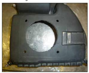
31. Drill the four 5/16" holes with a 5/16" drill bit and the 4" hole with a 4" hole saw. Deburr the holes. Some cutting or grinding of the webbing on the inside of the lid will be necessary so the hardware will sit flat.
