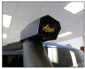
28. Install the Snorkel head onto the top of the snorkel and secure with the provided hose clamp. NOTE: During severe inclement weather AIRAID recommends installing the Snorkel head with the opening pointed towards the rear of the vehicle to prevent water, snow and ice from entering the intake system.
