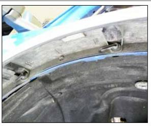
3. On vehicles equipped with extended fender flares, rotate the quarter turn fasteners counterclockwise to release and then remove the flare from the vehicle.
