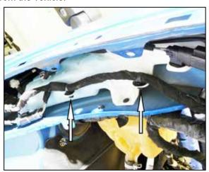
6. Unhook the wiring harness from the washer bottle
