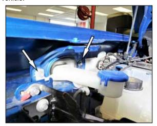
5. Remove the two bolts that secure the windshield washer bottle filler neck and remove the filler neck from the vehicle.
