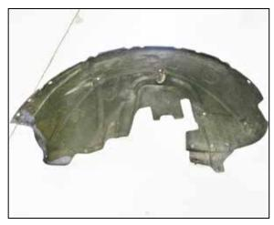
4. Remove the fasteners that secure the inner fender and then remove the inner fender from the vehicle.
