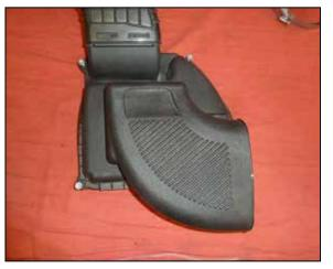
33. Secure the snorkel adapter to the lid using the provided bolts and thread locker.
