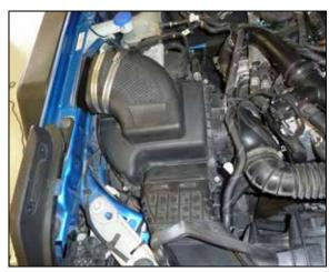
35. Install the lid back onto the air filter housing and secure with the factory hardware. Removing the rear housing mounting bolt will allow easier access the rear/fender side bolt. Once the bolts are tight, resecure the air filter housing with the factory bolt.
