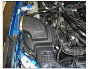
36. Slide the coupler hose onto the snorkel adapter and secure with the provided hose clamps.
