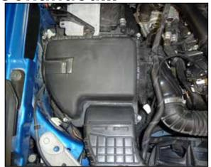
29. Remove the factory air filter housing lid.
