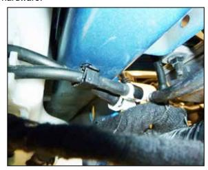
26. Reconnect the washer hose connection and secure the hoses with the factory clip.
