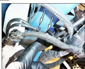
7. Disconnect the windshield washer hose at the union fitting and then unhook the mount from the inner fender.
