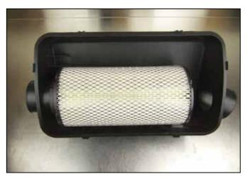
NOTE: the Airaid RZR 1000 Air Filter is installed in the air box differently than the OEM filter.
