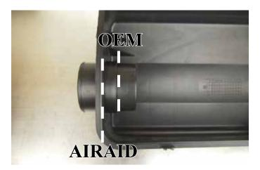
1. Notice the two stops on the mounting tube inside the air box. The first is the stop location for the OEM filter. The second stop, at the wall of the air box, is to be the Airaid stop.
