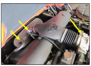
**8.** Re-secure the intake tube onto the throttle body and re seat the grommets on the radiator shroud posts. Re connect the MAF and air pump breather line.
