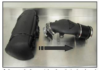
**2.** Separate the factory air box from the intake tube and Air Flow meter.
