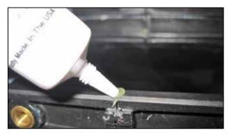
1. Using supplied grease; apply 2 separate beads of grease in the area shown.
