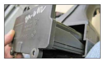
3. With filter inserted into frame, insert assembly into air box.
