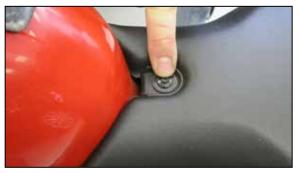
1. Loosen the allen screw shown and remove the seat.
