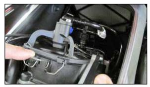
10. Unclip front and rear shrouds and remove as one unit. (fig 10)
