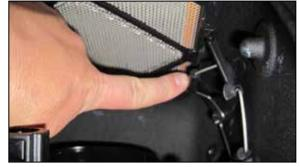
11. Pull bars down to release air filter cage & filter then wipe out any dirt or debris from the air box.
