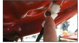
7. Disconnect fuel line under fuel tank. WARNING: Some fuel will spill out; have a rag ready to absorb any spillage.
