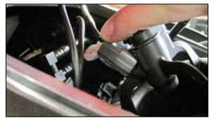
8. Disconnect front and rear injector connectors.
