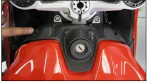
3. Remove the four allen screws shown and remove ignition cover above fuel tank.
