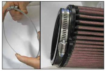
5. Squeeze the clamp supplied with the K&N® filter as shown to conform to the filter base flange and Install hose clamp onto air filte
