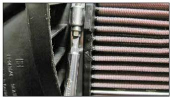
9. Re-position clamp to ensure correct placement onto flange of K&N<sup>®</sup> filter and tighten.
