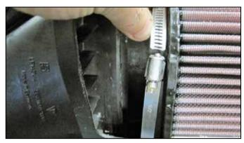
7. With filter resting in air box, loosen clamp completely from the air filter. Filter cannot be installed with the clamp tightened onto air filter flange.
