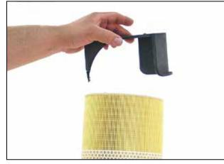
3. Remove the dirty air filter and remove the screw (which will not be re-used) that fastens the top plate to the filter and depress the four tabs to release the top plate from the filter.
