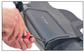
11. Install air filter cover and fasten screws.
