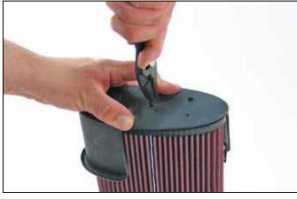
4. Install the top plate from the OE filter onto the K&N<sup>®</sup> filter. Using a pair of pliers, pull the rubber tip from the K&N<sup>®</sup> filter through the hole on the filter top plate.
