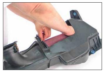
6. Place K&N<sup>®</sup> filter top side first into air box. NOTE: make sure that the filter lid is orientated correctly so that the screw hole is reused on step 9. Position filter so that it can be pulled toward air box flange.
