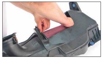
8. Slide filter onto flange portion of OE air box. You may be required to place one hand on the top of the filter and push. Use pull tabs built into filter base to assist pulling filter flange onto air box flange until filter is seated.
