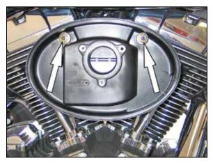
4. Remove the two crank case breather bolts securing the filter back plate and remove the back plate.
