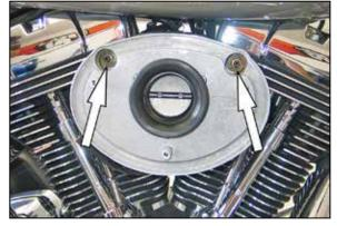
7. Install the filter back plate onto the throttle body and secure with the factory breather bolts and throttle body bolts provided.
