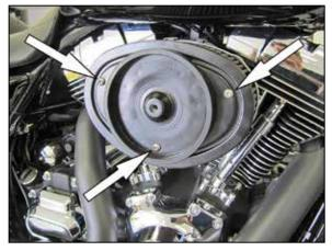
8. Install the K&N $^{\odot}$  air filter onto the back plate and secure with the provided hardware. NOTE: Be sure to place one drop of thread locker onto each bolt.
