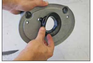
5. Install the provided intake venturi and three throttle body bolts into the K&N<sup>®</sup> back plate.
