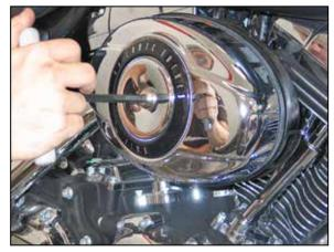
2. Remove the bolt securing the air filter bonnet
