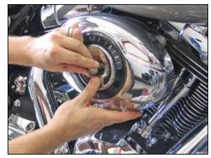
10. Install the bonnet onto the K&N<sup>®</sup> air filter and secure with the factory bolt.
