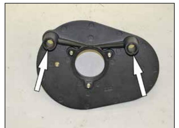
7. Install two of the provided O-rings into the crank case breather plate as shown.
