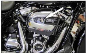
2. Loosen and remove the bolt which secures the decorative filter cover and remove the cover from
