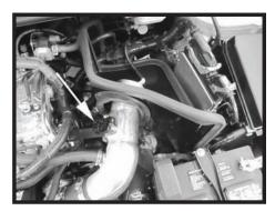
Step 17 Route the MAFS wire harness through the heat shield opening next to the intake tube and then connect the electrical connector to the MAFS.
