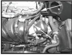
Step 11 Install the "L" shaped bracket and fasten it securely in place using the hardware removed on Step 8. Install the reducer coupler on the throttle body and fasten securely. Install the second clamp but do not tighten at this time.
