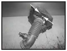
Step 12 Remove the two screws that secure the MAFS to the factory air box and remove the MAFS.
