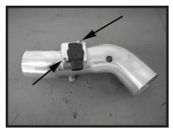
Step 13 Install the MAFS into the Spectre Performance intake tube and secure with the supplied screws.
