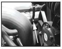
Step 8 Using the supplied hardware, install the "L" bracket onto the frame using the hole that is threaded. This is located towards the front of frame on the driver's side.
