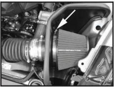
Step 12 Install the filter and securely fasten to the velocity stack adaptor.
