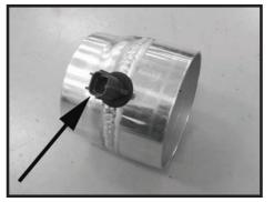
Step 5 Install the supplied grommet into the intake tube and then install IAT sensor into the grommet.
