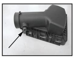
Step 4 Turn the IAT sensor counterclockwise and remove it from the factory intake tube. Remove the O-ring from the sensor.
