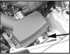
Step 3 Remove the factory air box by removing the 10mm bolt and lifting it out.
