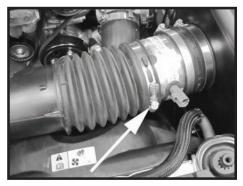
Step 10 Align the new intake tube with the factory intake tube and once in position fasten the tube securely in place.
