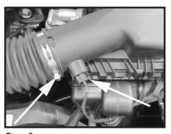
Step 2 Disconnect the electrical connector on the Intake Air Temperature (IAT) sensor. Loosen the clamp from the intake tube to the air box lid.
