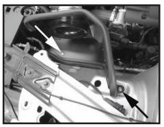
Step 9 Install the heat shield and secure it using the supplied hardware. Fully tighten all mounting hardware.
