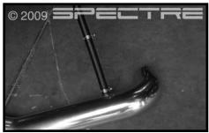
Step 11 Install the supplied breather hose onto the Spectre intake and secure with the supplied clamp. Install the second clamp onto the hose, but leave loose at this time.
