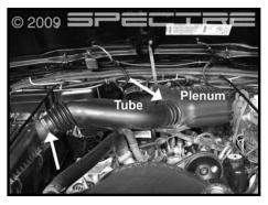
Step 2 Loosen the two hose clamps on the stock intake tube and remove the tube.
