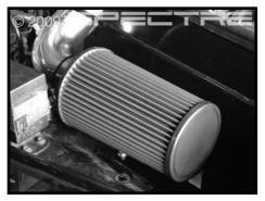
Step 14 Install the Spectre air filter onto the intake tube. Fully tighten the clamp.
