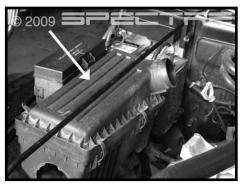
Step 4 Remove the air box lid and filter element.
