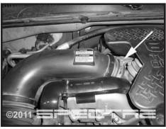
Step 3 Using a 5/16" nut driver (or flat blade screwdriver), loosen the clamp at the turbo.
