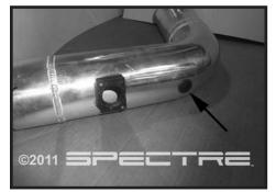
Step 7 Install the grommet in the intake.
