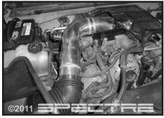
Step 13 Install the intake tube into the vehicle, position it as shown and once tube is in desired location fasten securely.
