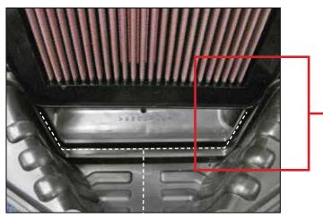
Fig. 1 Sealing Groove in air box
